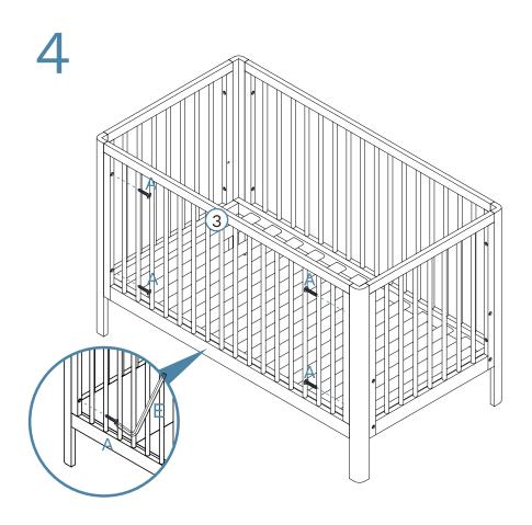
Attach panel [3] to assembled frame as shown and secure with  $4\ x$  screws (A). Tighten with an Allen Key (E).
