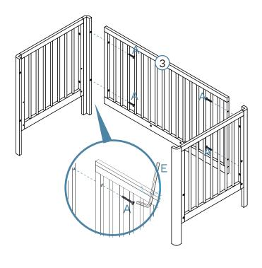
Attach assembled panels together with panel [3] and secure with 4 x screws (A). Tighten with an Allen Key (E).
